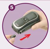
Press the cap back on to the lancing device. The cap snaps in to place with a click.
