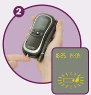
Hold the meter so the test strip is pointing downwards. Touch the drop of blood against the front edge of the test strip where the black notch is located. The test strip draws up blood.
