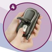
Insert new test strip drum.
