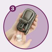
Tip the meter forwards, the test strip drum drops out.
