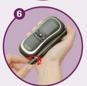
Twist the cap to the desired depth setting (11 settings in total).
